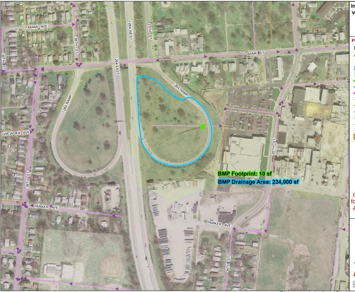
Ohio River Sewershed Solution ID # L\_OR\_MF\_019\_S\_12\_A I-264 On-Ramp Dry Well
