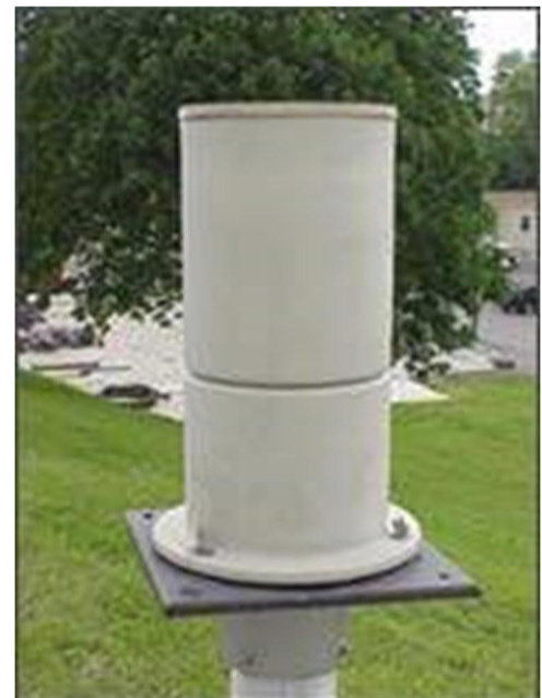
Figure 2.2-3 Typical Rain Gauge
